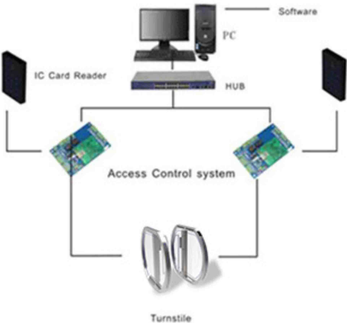
Access Control System
